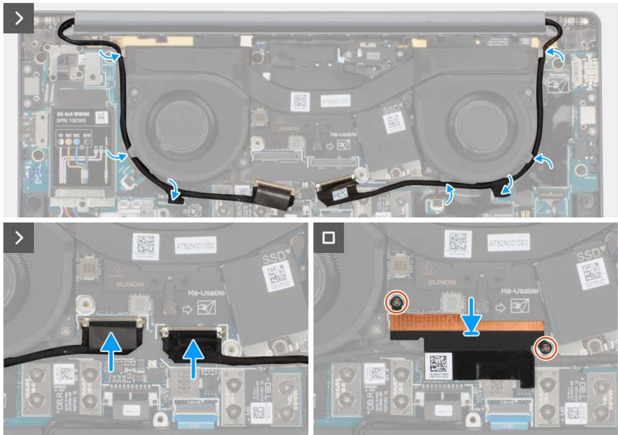
Figure 60. Connecting the display and camera cables
