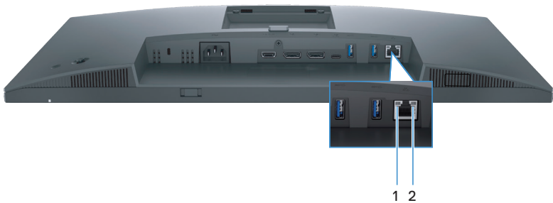
Figure 10. RJ45 connector LED status
