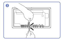
Insert the appropriate cable into the hole from which the silicone bar was removed.
